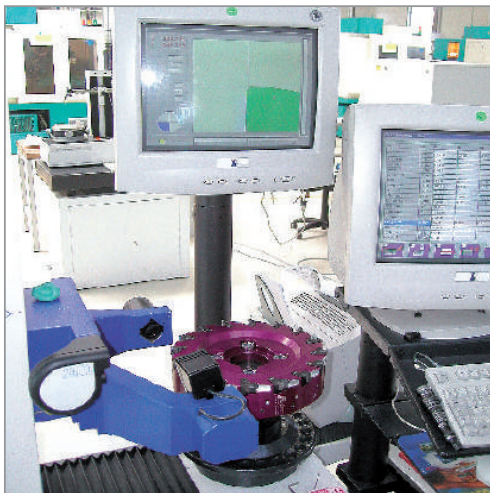
Measure machine for cutting edge adjustment.
